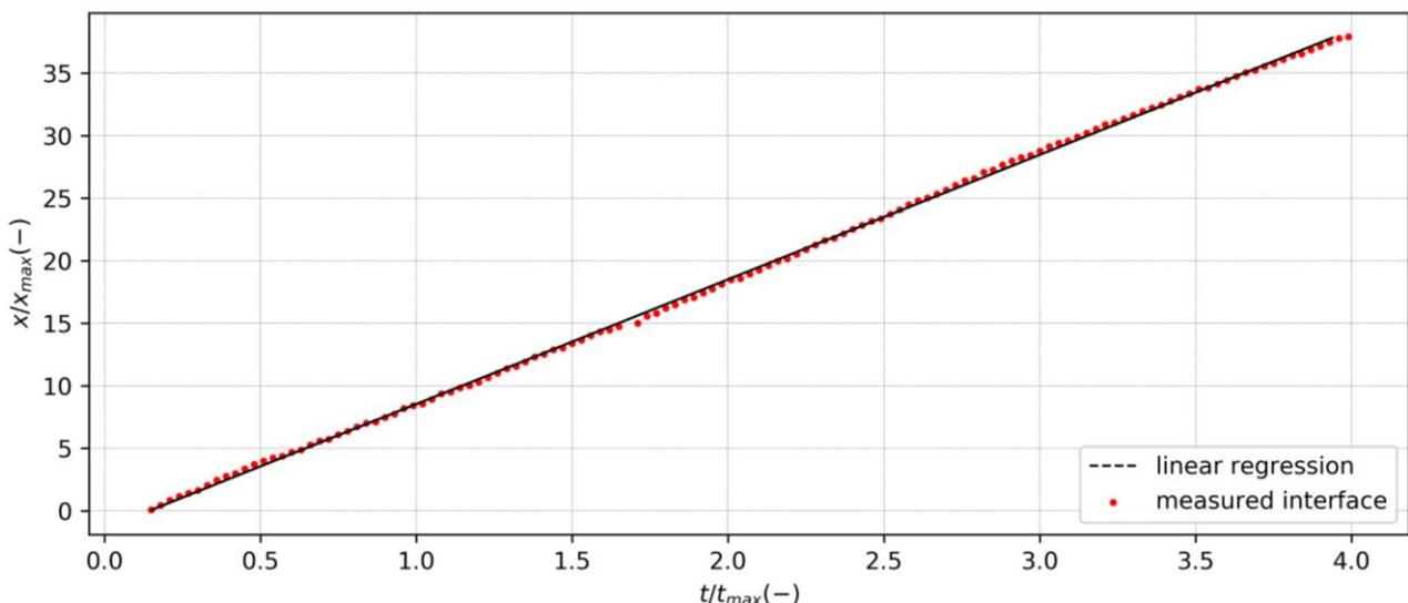
Figure 3 - Time evolution of the gravity current front location. x- and y-axis are normalized by the time and special scale of the erodible bed
