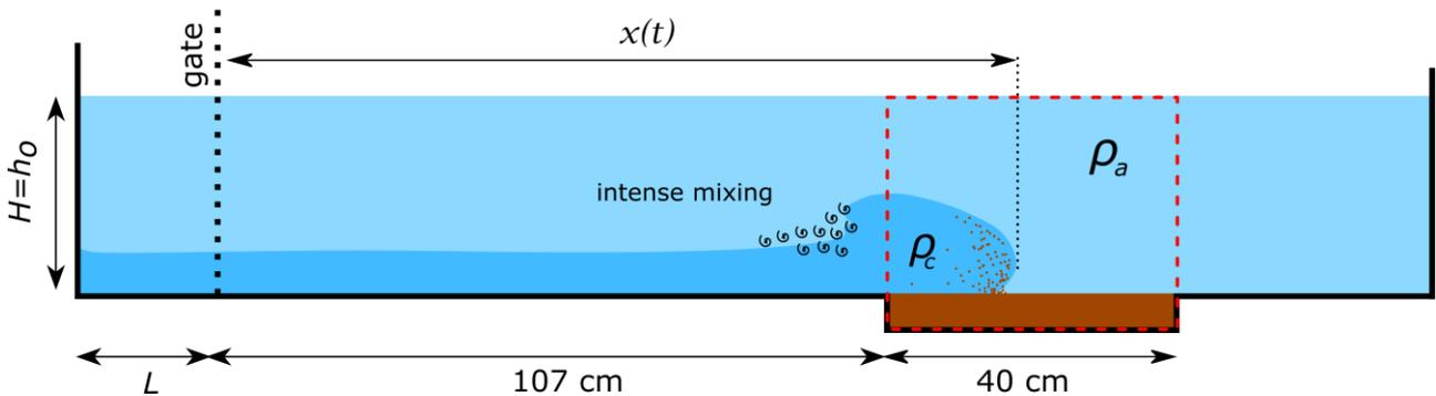
Figure 1 – Side view of the experimental set-up. Red dashed box indicates the region where video was recorded.
