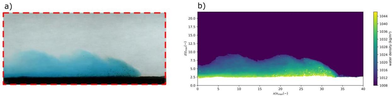
Figure 2 - Gravity current flowing under the erodible bed ( $x = 154$  cm). a) snapshot from video and b) digitalized image processed by the Dynamic.
