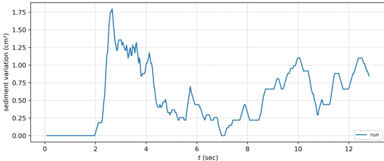
Figure 5 - sediment resuspension observed at 140 cm from the left-hand side end of the tank.
