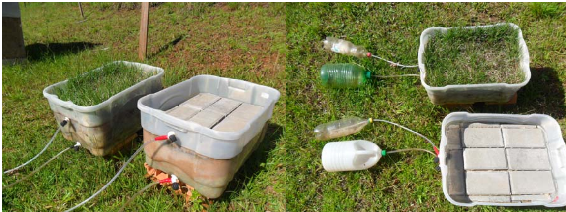
Figure 4: the lysimeters installed in environment.
