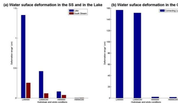
Fig. 7: Wind impact on the WSD in the FP: a) over the lake and the SS b) in the CC
