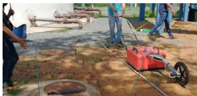
Figure 2: Photo of GPR data collection on surface feat 200 MHz antenna. Source: Authors, 2021.
